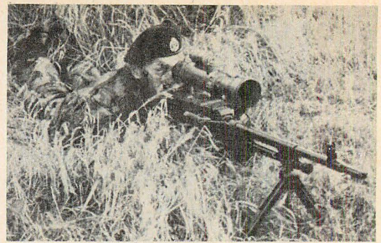
Tri-lite (G. Britain) sight on FN/MAG 7.62 LMG.
